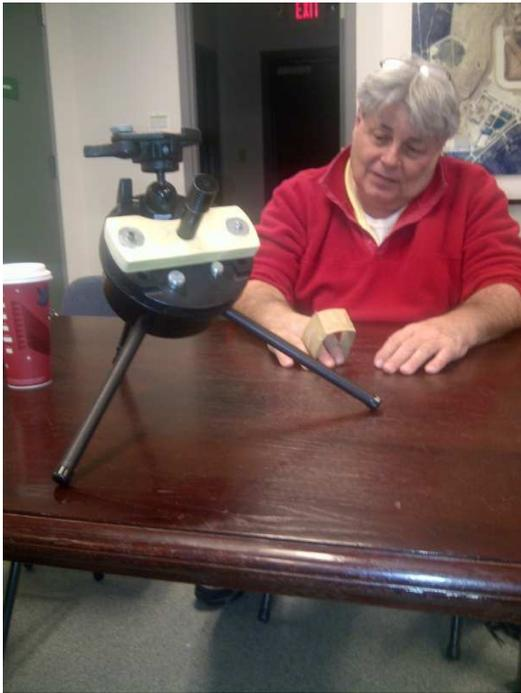
Club raconteur Steve Boerner demonstrating his tracking mount fashioned from an old, cheap, plastic SCT. With one piece of scrap wood and a camera tripod head he's converted this to a perfectly suitable mount for widefield astrophoto work.
