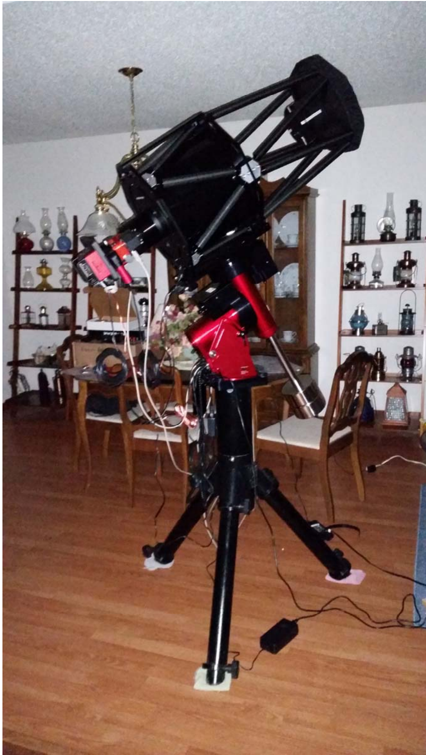
Software Bisque Paramount MX+ with an Astronomy Technologies 12" Truss RC. Owned by Dan Crowson and friends. Dan will provide a talk at an upcoming monthly meeting.
